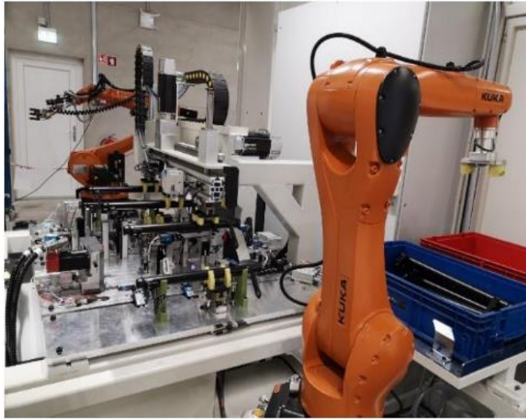
Figure 13: Automated visual inspection system (Bračun & Lekše, 2019)
