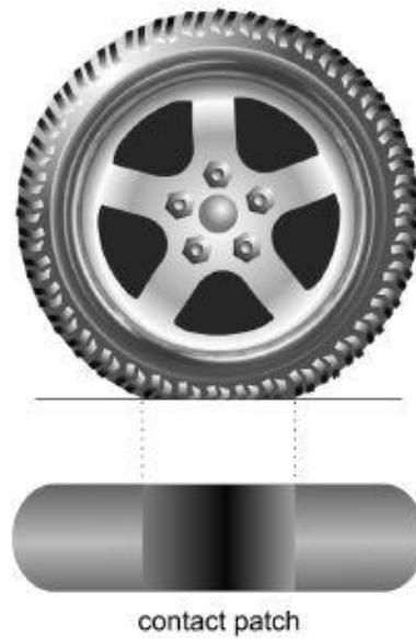
Figure 2.6: Tire to the vertical load of the vehicle deforms (Rajamani, 2012)
