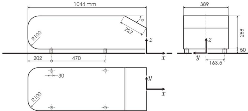
Figure 2.1: Dimensions of Ahmed Body. (Guilmineau et al., 2016)
