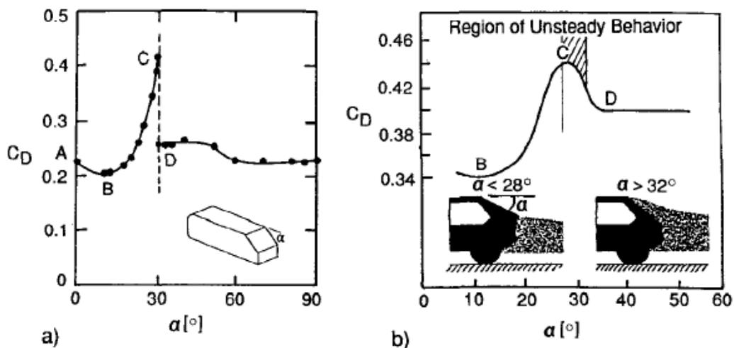
Figure 2.2: Dependence of drag,  $C_D$ , on the slant angle  $\alpha$  of the upper-rear surface of fastbacks, and the existence of a critical phenomenon: (a) simple body, (b) automobile. (Hucho & Sovran, 1993)
