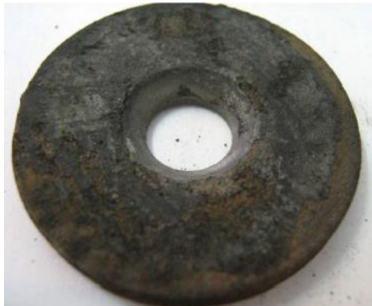
Figure 2.1: Uniform corrosion on disc coupon (Mansoori et al., 2017)
