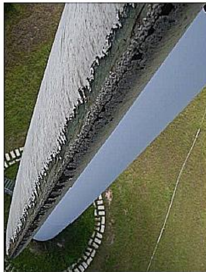
Figure 1.3: Leading edge erosion of a rotor blade (J. Liersch & J. Michael, 2014).
