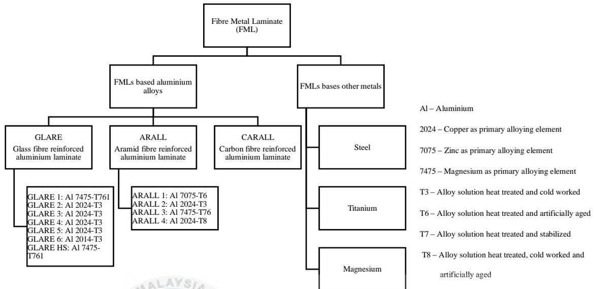
tolerance material (Zhen, 2015). The common metals that are been used to fabricate fibre metal laminate are aluminium, magnesium, or titanium and the common composite reinforcement are glass fibre, carbon-fibre, or kevlar. Figure 2.1 shows the type of FML's that had been developed base on its metal and reinforcement.
