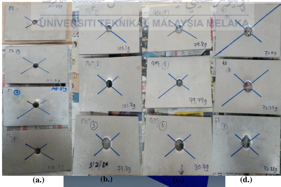
Figure 4.1 shows the perforated FML,s for the four stacking sequence.
