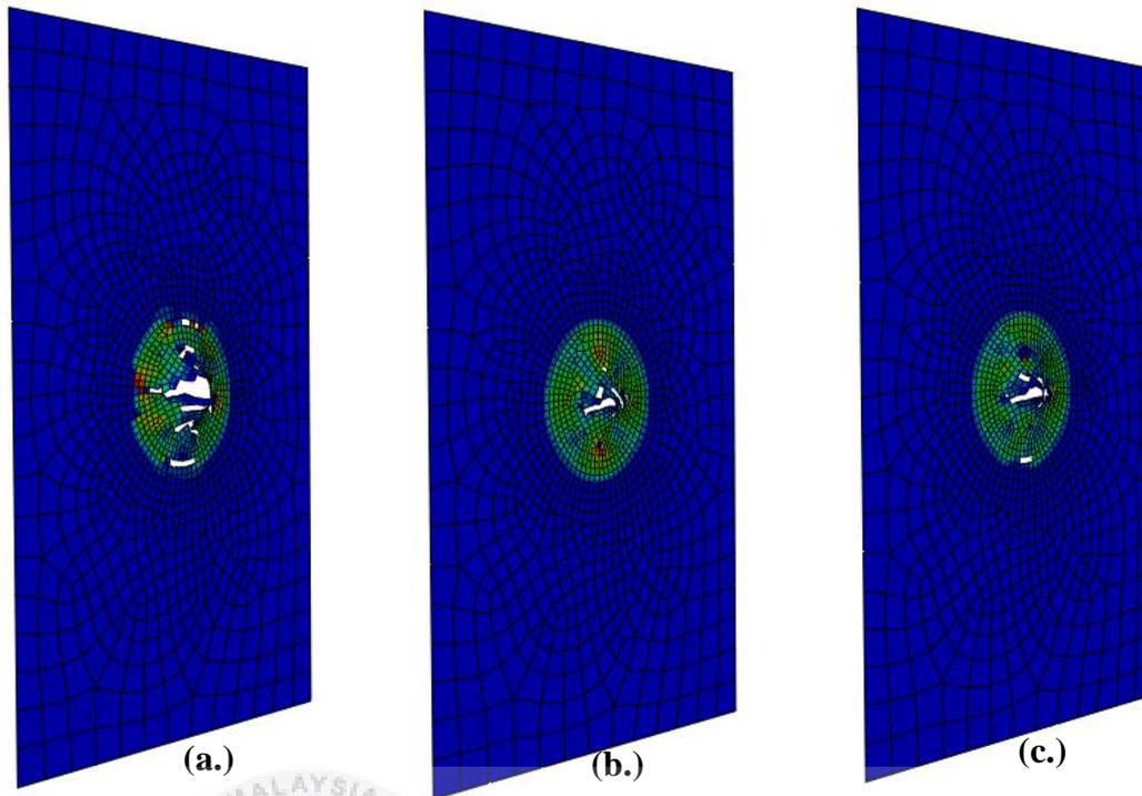
Figure 4. 11: Energy heat map of the fibre glass/epoxy. (a.) 0.5 mm, (b.) 1.0 mm, (c.) 1.5 mm.
