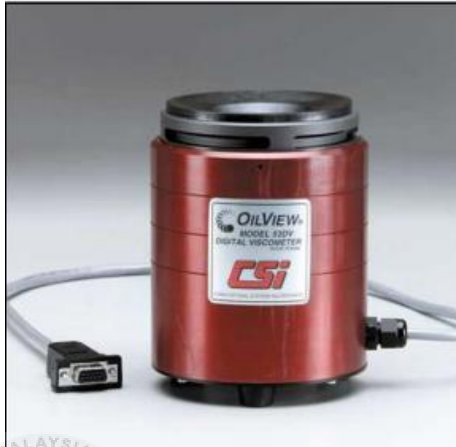
Figure 3.2: 52DV model for viscosity test
