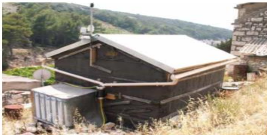
Figure 2. 4: Dew collector with thermal isolated polycarbonate plate from Muselli et al.
