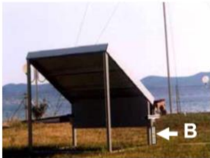
Figure 2. 3: Design for dew collector with angle 30 degree
