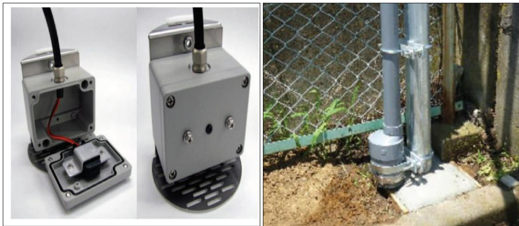
Figure 2. 4: Pressure-sensitive device measure the water level
