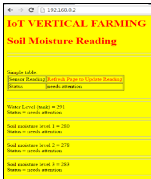
Figure 2.3: Interface of the status, soil moisture level and water level tank
