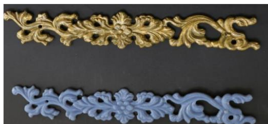
Figure 2.3: Top figure shows the painted model and the bottom figure shows the printed model (Shui et al., 2016)
