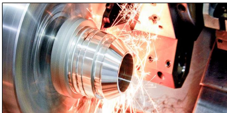
Figure 2.2: Example of dry turning process
