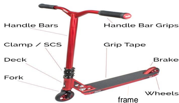
Figure 2: Basic part in Scooter
