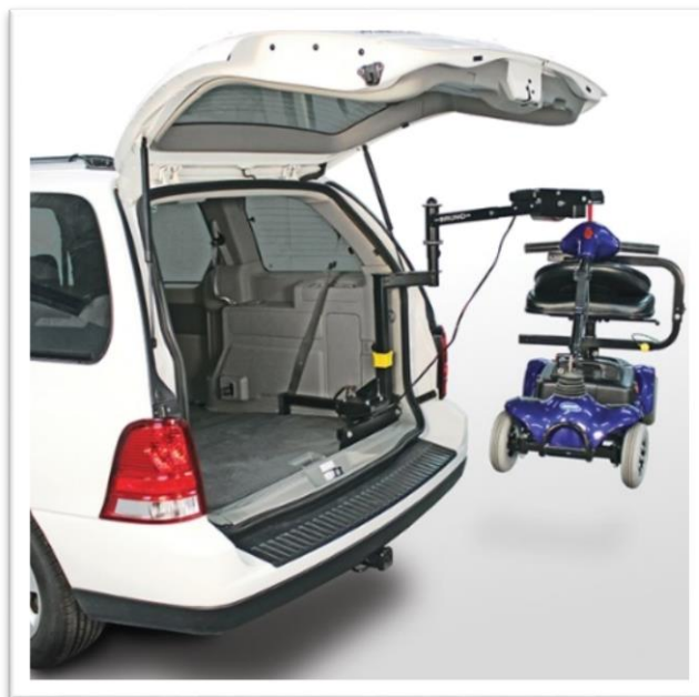
Figure 2.4: Wheelchair Lift for trunk vehicles (James, 2012)
