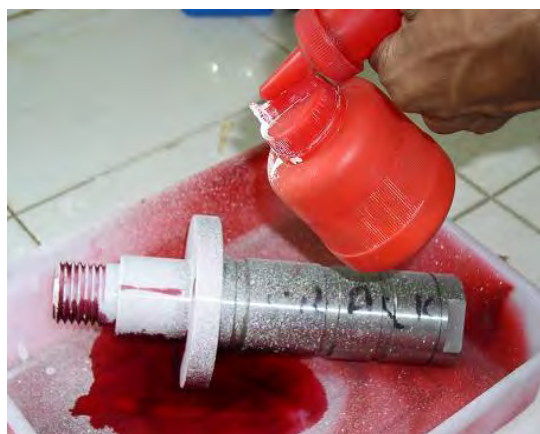
Figure 2.1: Penetrant Test Material is sprayed on Test Sample [3]
