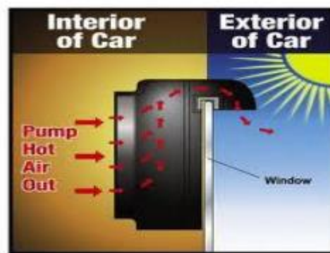
Figure 2.5: Mechanism for reducing temperature.(M.F. Basar, M. Musa, M.Y. Faizal, 2013)
