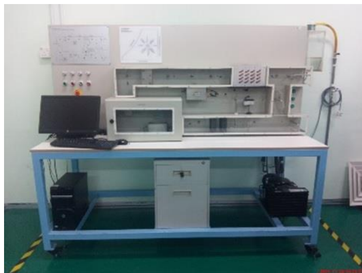
Figure 2.2 : Recirculation Air Conditioning Equipment
