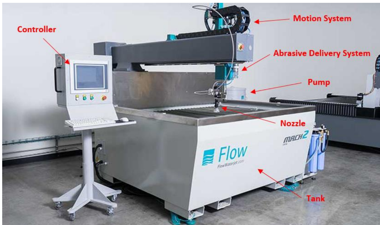
Figure 2. 1 : Component of abrasive waterjet machine.
