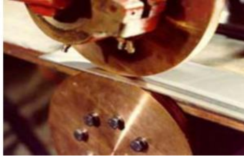
Figure 2.4 RSEW producing continuous joint (Devarasiddappa., 2014)
