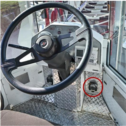
*Figure 1.1 Position of Dead Man Switches on a lorry. Reprinted from (“Tiller Deadman switch — tractor-drawn aerial,” n.d.) retrieved from <http://www.tractordrawnaerial.com/tiller-deadman-switch>*
