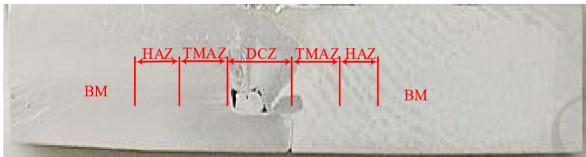
Figure 2.9: Zones formed in FSW joint performed (Cetkin et al., 2019)
