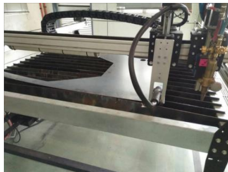
Figure 4.2: Cutting process by using the CNC plasma cutting machine for mild steel sheet with thickness of 0.8 mm.
