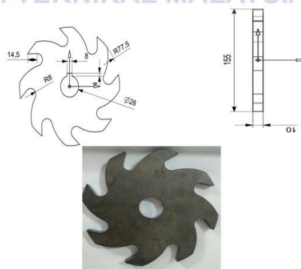
Figure 2.12: Design of the blade. (Pavankumar S. B. et al, 2018)
