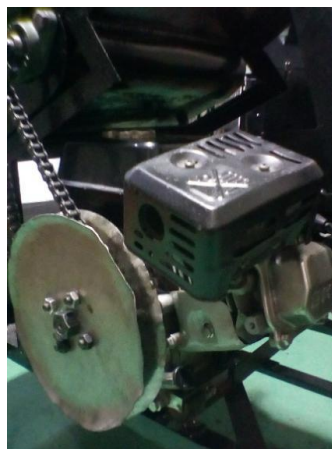
Figure 4.7: Petrol engine motor located at the lower side of the body frame.
