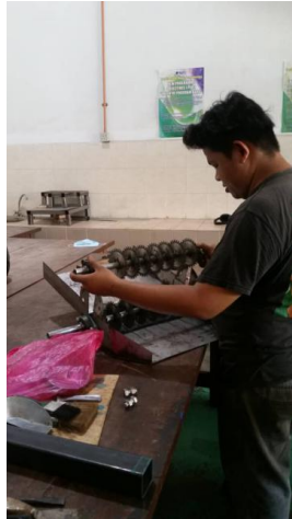
Figure 4.6: Assembly process of the upper and lower blade shafts on the casing blade.
