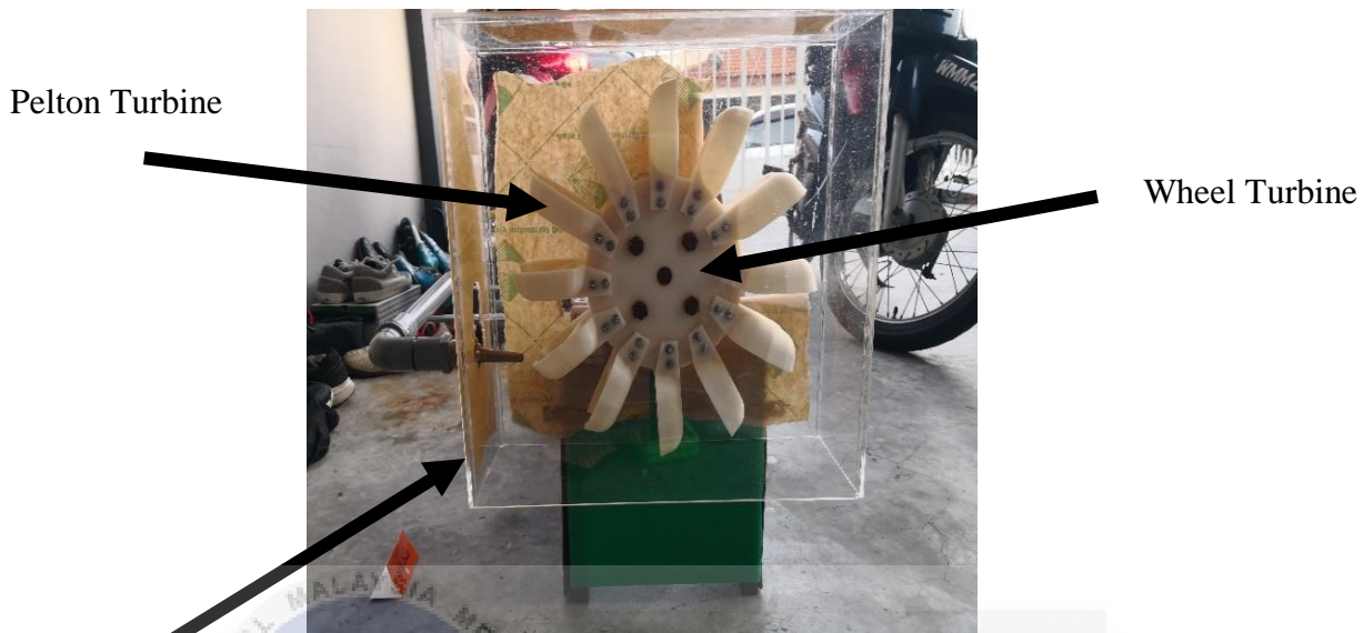
Figure 3.5: Front View of Pico Hydro Generation System
