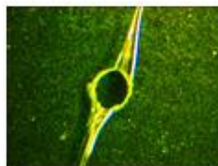
Figure 1.3: Chemically strengthened glass cracks when undergo conventional drilling process.
