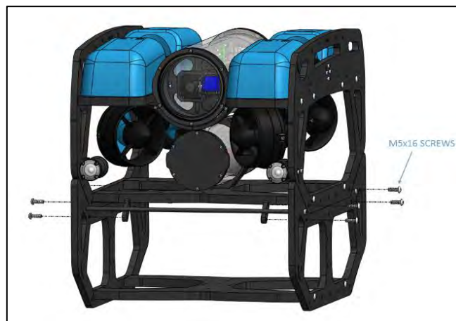
Figure 3.29: Payload Skid fit to the bottom of BlueROV2
