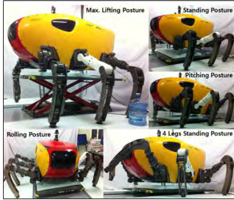
Figure 2.22: Posture change test by using 6 legs and 4 legs
