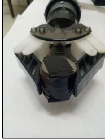
Figure 3.31: The load grasped by gripper (top view)
