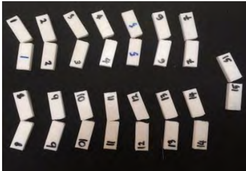
Figure 4.16: PLA specimen after impact test.
