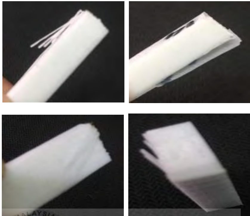
Figure 4.23: PLA material after impact test.
