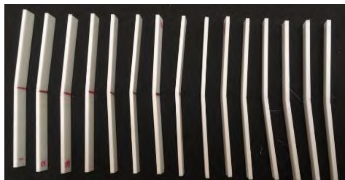
Figure 4.27: PLA specimen after flexural test.
