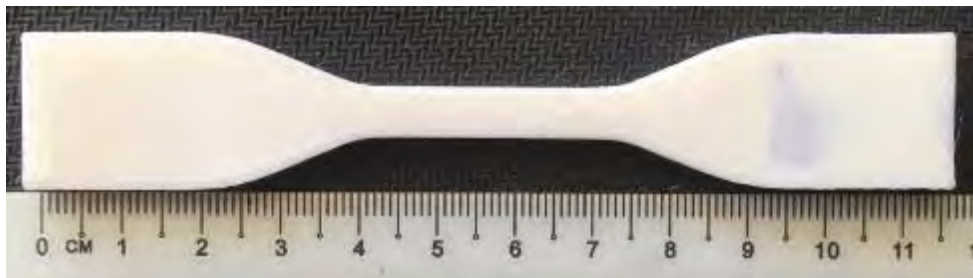
Figure 4.1: Tensile test specimen for ABS material.
