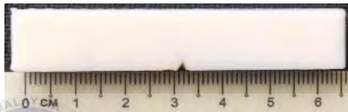
Figure 4.14: Impact test specimen for PLA material.
