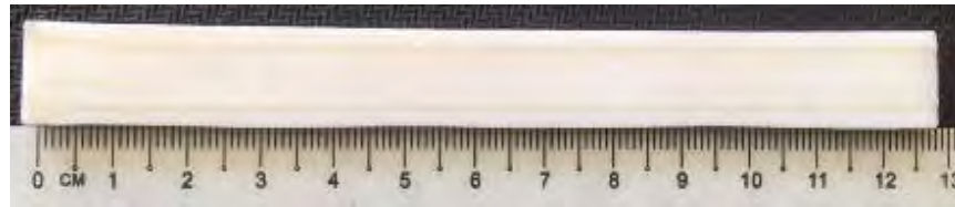
Figure 4.24: Flexural test specimen for ABS material.
