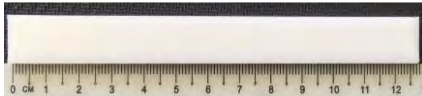
Figure 4.25: Flexural test specimen for PLA material.
