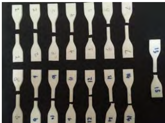
Figure 4.3: ABS specimen after tensile test.
