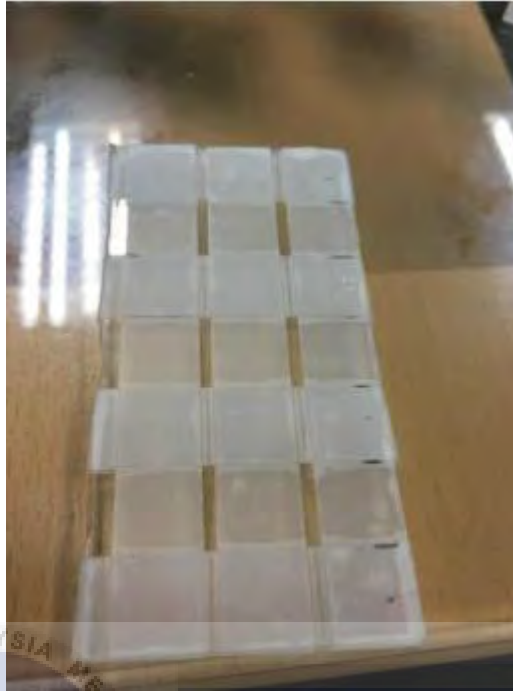
Figure 3.11: Acrylic plate after layered with Scotch Tape.
