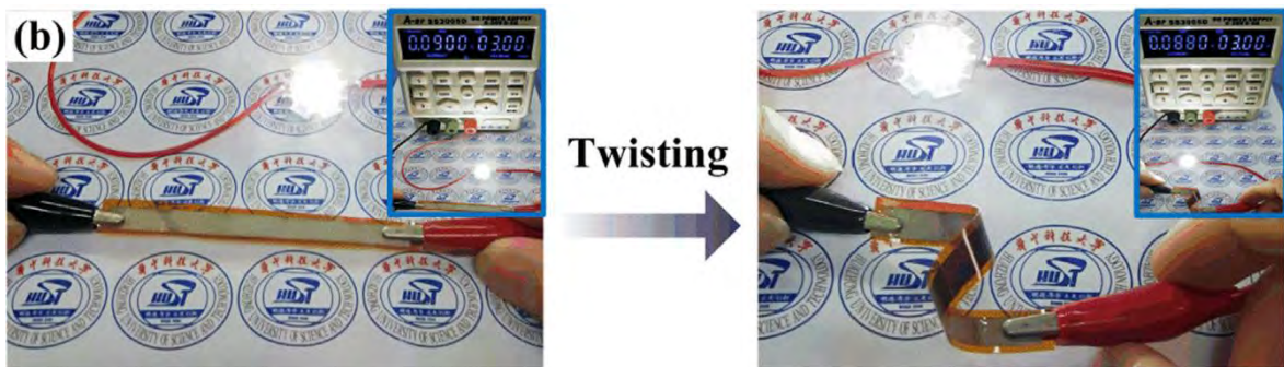
Figure 2. 7 Cyclic twisting load experiment (Mou et al, 2018)
