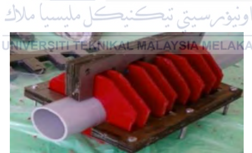
Figure 2.10 : Four pole linear stator (Sahin and Ozdinc, 2014)
