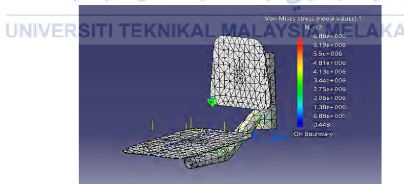
Figure 6.7: Von Mises Stress of Seat using Mild Steel (Source: Author)
