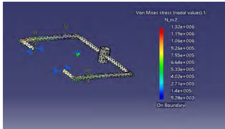
Figure 6.19: Von Misses Stress for Handle Bar with 50N using Stainless Steel
