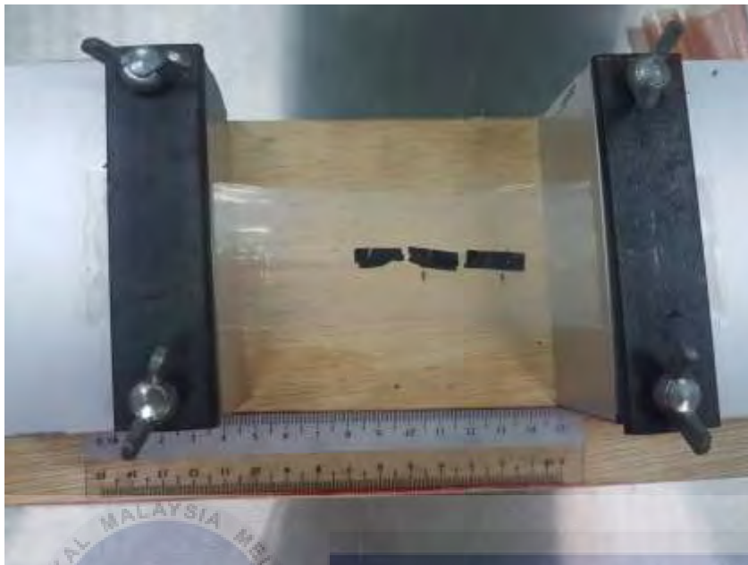
Figure 4.5 crack of 100 wt% conductive ink on TPU after tensile test
