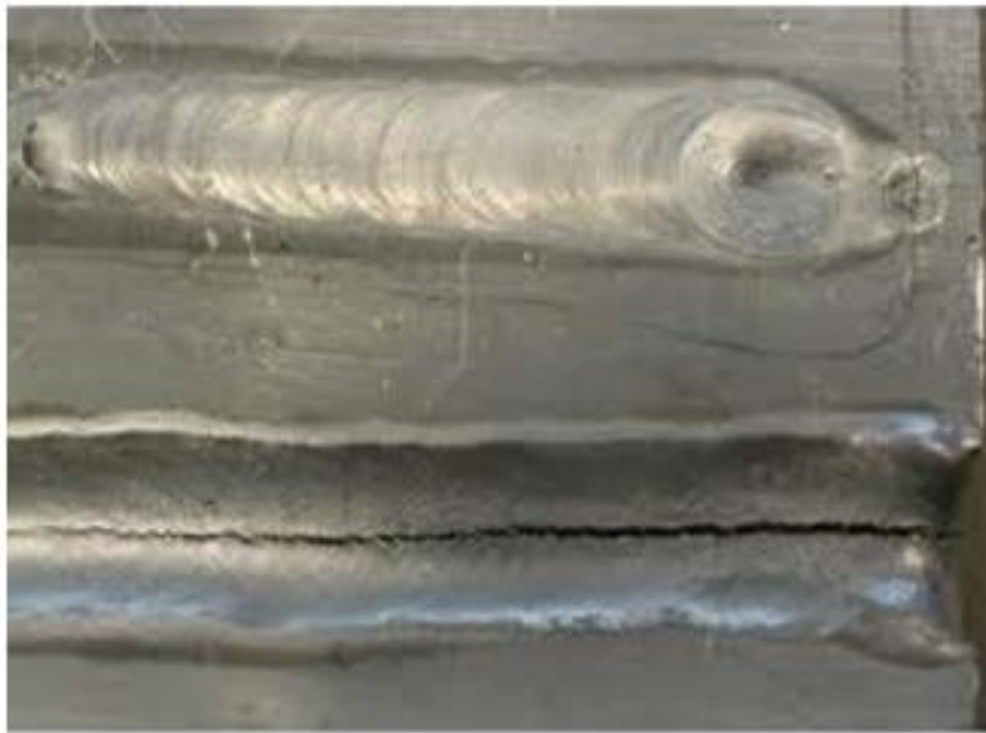
Figure 1.4: Solidification cracking (Chandra and Vivekanand, 2013)
