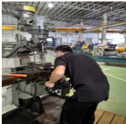
Figure 1.3 User bends his back to have a clearer view on the work piece.
