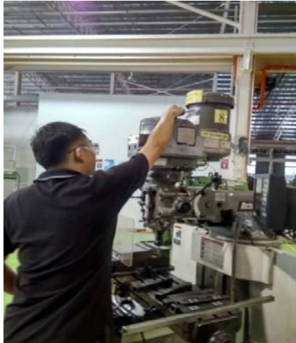
Figure 1.2 User trying to tighten or loosen the draw bar with a spanner
