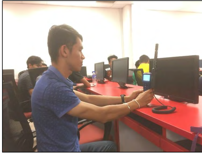
Figure 3.6: Measurement of Temperature, CO 2 and Relative Humidity conducted at MB1, ground floor of PBPI building using a TSI Indoor Air Quality meter.
