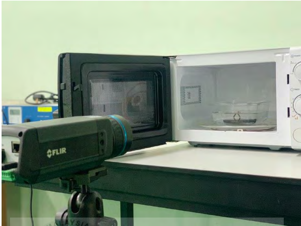
Figure 3.4: The plasma generation in liquid set up.
