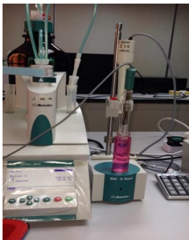
Figure 3.12: Calibration process using buffer solution
