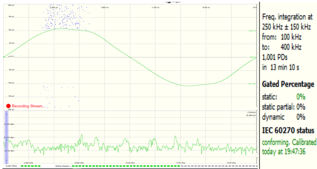
Figure 4.9: 1000 electrical discharges of Fresh Midel eN oil
