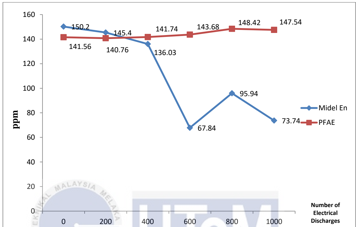
Figure 4.15: Moisture of fresh Midel eN and PFAE oil
