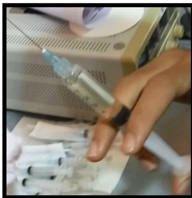
Figure 3.6: Syringe tube fill with natural ester oil.
