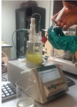
Figure 3.8: Filled NE1 sample into Coulometric Karl Fisher Titration tube.
