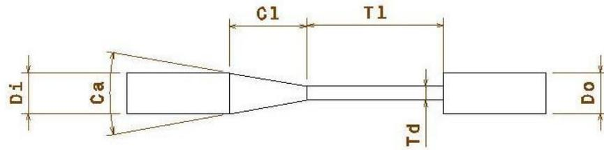
**Figure 3.2:** The dimension of the nozzle
