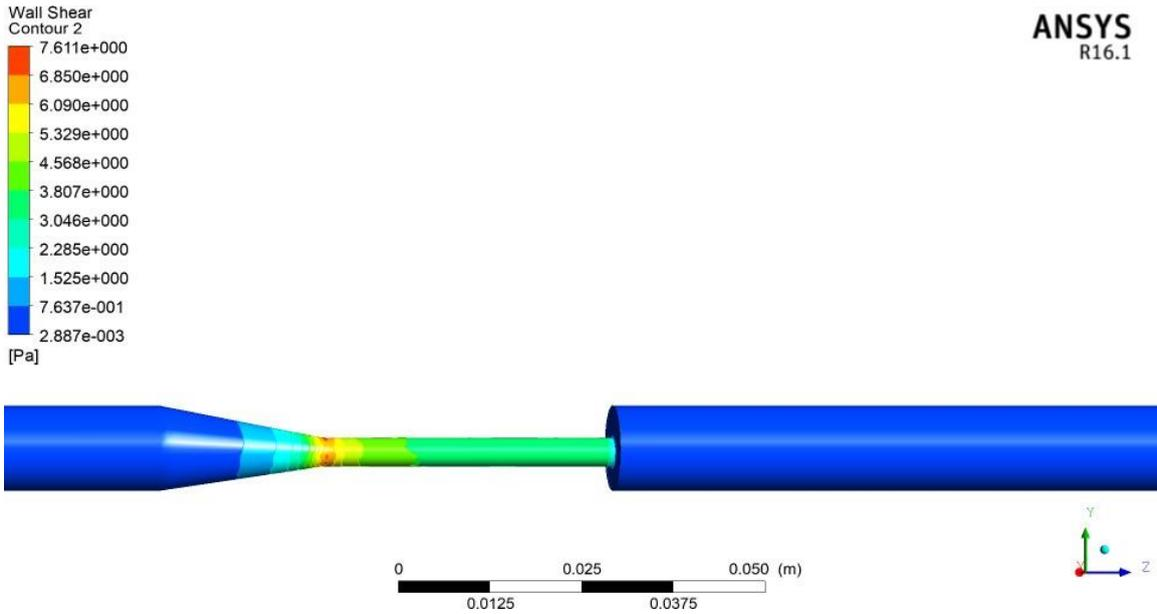
Figure 4.13: Contour for wall shear stress Non-Newtonian model Carreau-Yasuda
