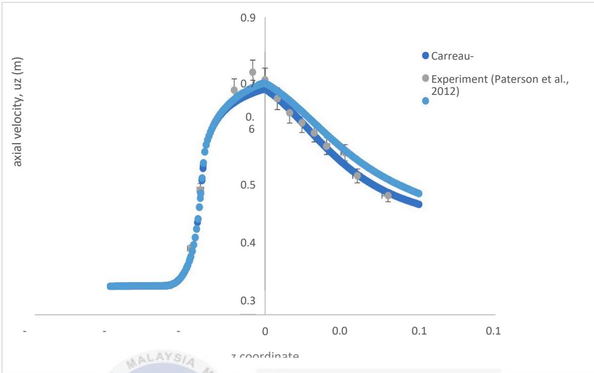
**Figure 4.5:** Axial velocity along the nozzle centreline for two different viscosity and experiment.
