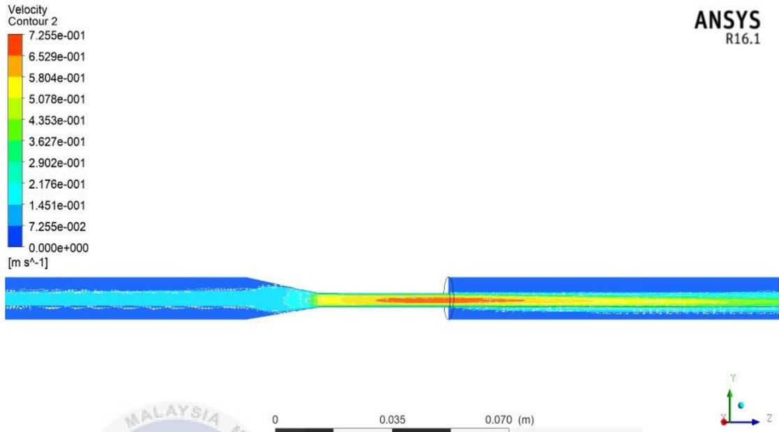
**Figure 4.7:** Velocity contour along the nozzle centreline for non-Newtonian Carreau-Yasuda viscosity
