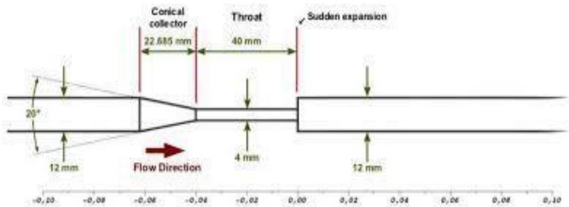
**Figure 3.4:** Specification for nozzle geometry (Min et al., 2014)
