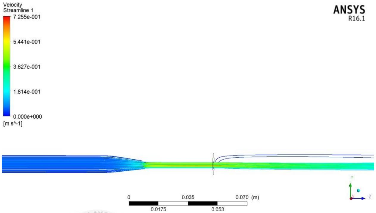
**Figure 4.9:** Streamline velocity for non-Newtonian model Carreau-Yasuda viscosity model
