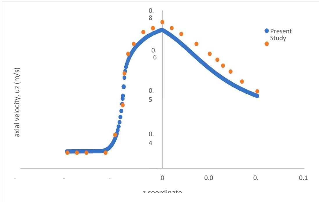
**Figure 4.2:** Axial velocity along the nozzle centreline for the present study and (Min et al., 2014) for Carreau-Yasuda
