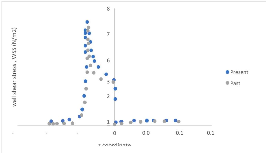
**Figure 4.3:** Wall shear stress of the axial position of the present study and (Min et al., 2014) for Newtonian
