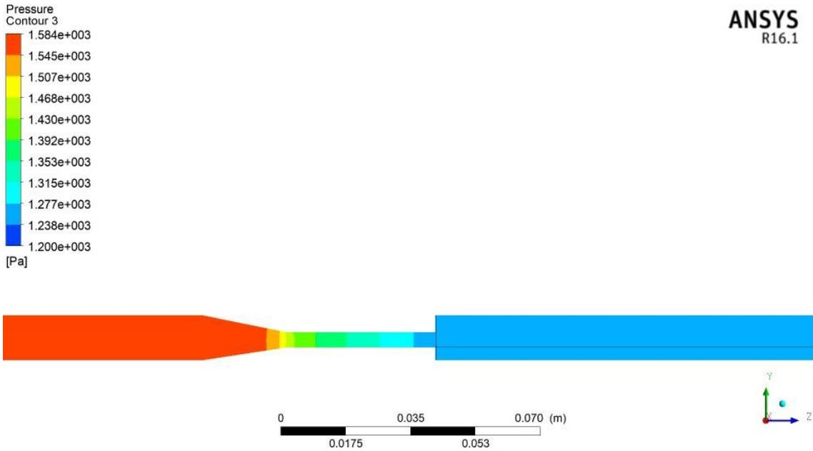
Figure 4.10: Contour for pressure Newtonian viscosity model
