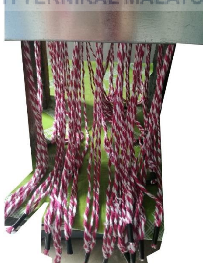
Figure 3.11: Wet string evaporative cooling system after modification
