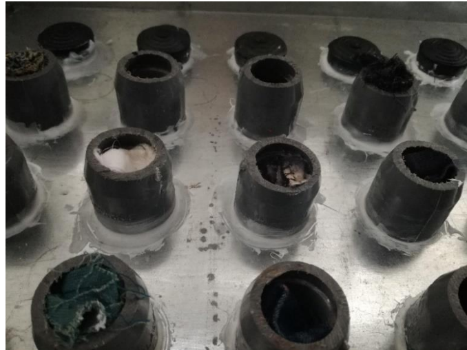
Figure 3.9: Wet cylinder with silicon sealant
