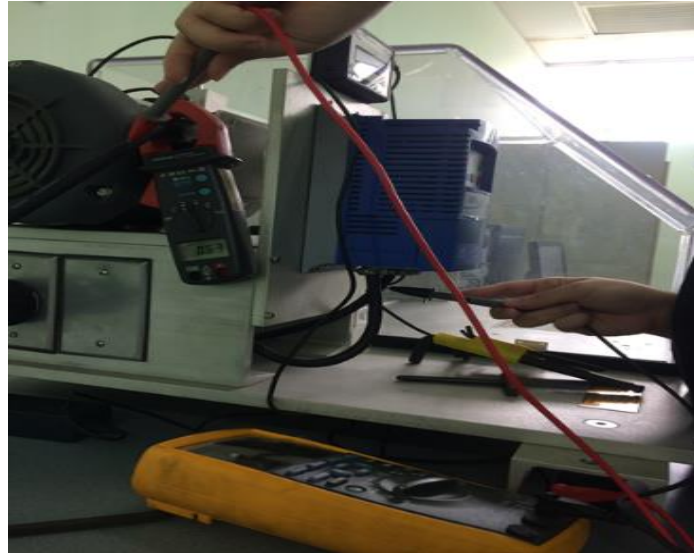
Figure 32 How the ammeter clamp and the multimeter is used on the MFS
