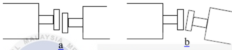
Figure 2 (a) Parallel Misalignment (b) Angular Misalignment
