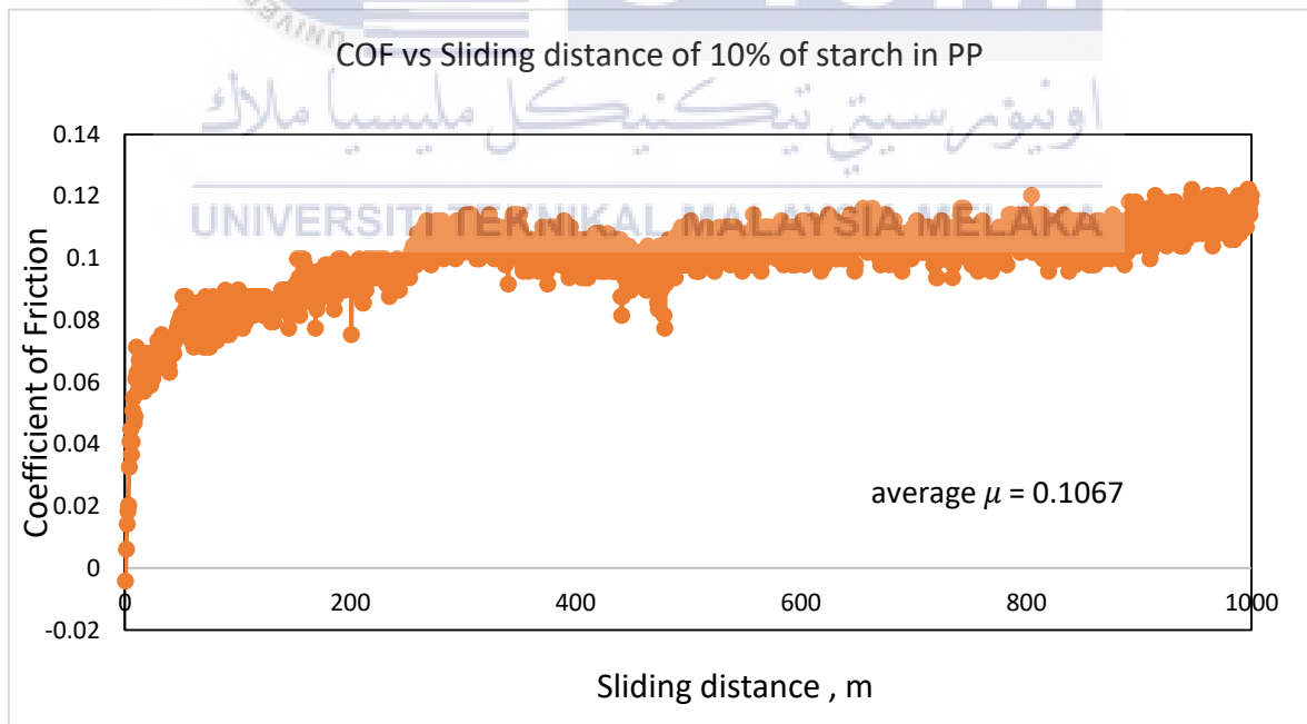
Figure 4.4: The Effect of 10% Tapioca Starch on COF of PP Composite Against Stainless Steel Ball
