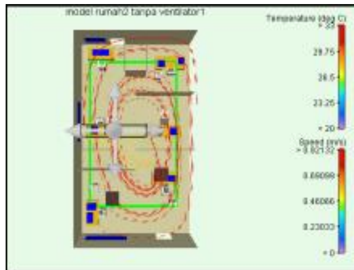
Figure 2.10 Air movement before installing the Ventilator
