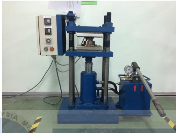
Figure 3.8: Hot press moulding machine for compaction process
