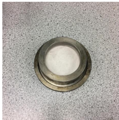
Figure 3.7: A 74x4 mm disc mould use for compaction process
