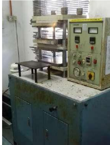
Figure 3.5: Motorise Hydraulic Molding Test Press Machine
