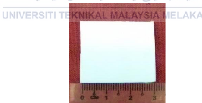
Figure 3. 4: Molded ABS preparation
