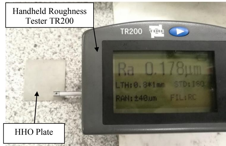
Figure 3.8: Surface Roughness Test with Handheld Roughness Tester TR200
