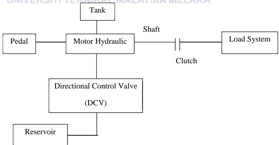
Figure 3.3: Functional of driveline propulsion system
