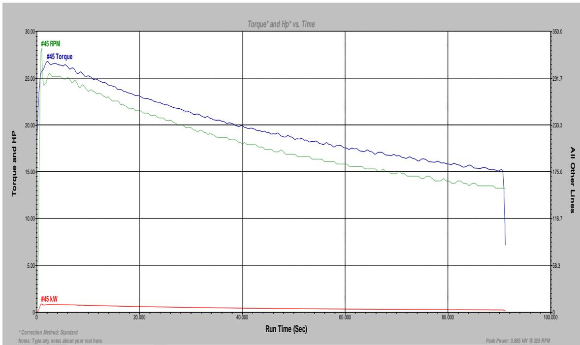
Figure 4.1: Torque and RPM vs. Run Time (Sec) for 200 bar with load 10 Nm
