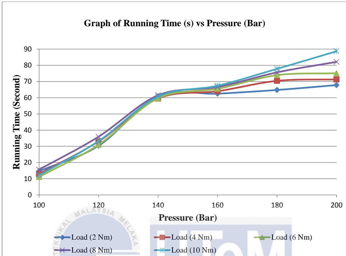
Figure 4.5: Effect of accumulator pressure different and running time
