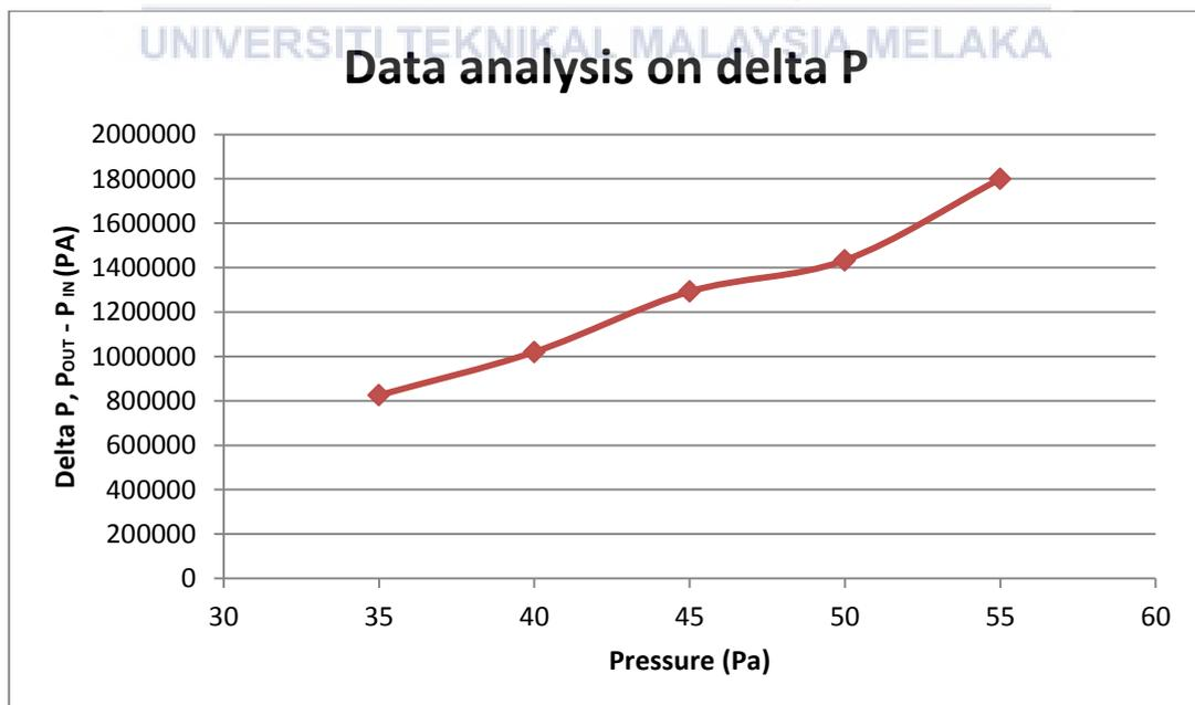
Figure 3.10: Pressure sensor calibration data analysis on delta P (Pa)
