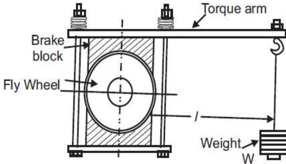
Figure 2.2: Prony brake dynamometer (G.G. Liversidge, K.C. Cundy, J.F. Bishop, 1980)
