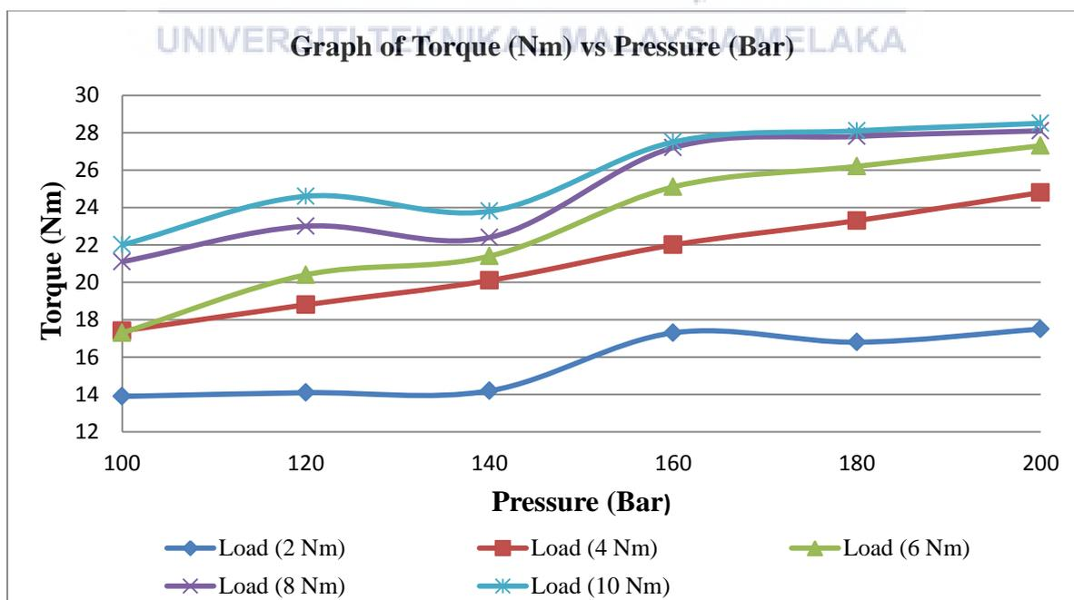
Figure 4.7: Effect of pressure changes to the torque
