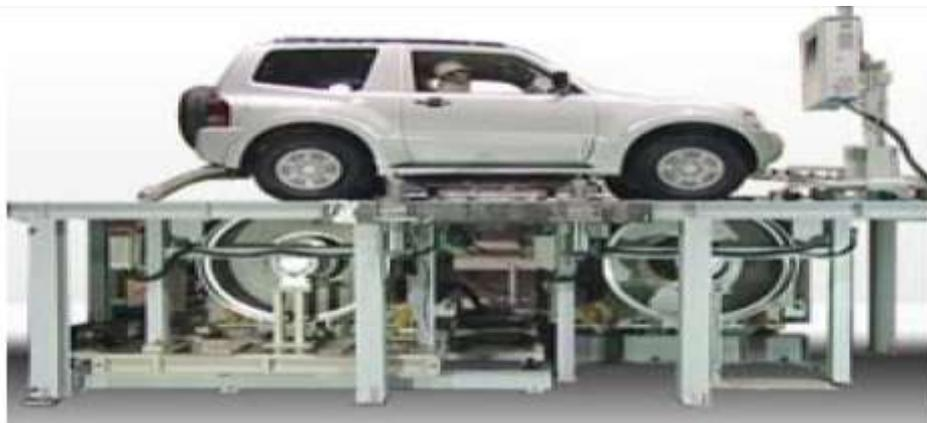
Figure 2.9: Conventional chassis dynamometer (Zhao *et al.*, 2013)
