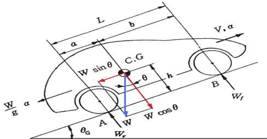
Figure 2.7: Vehicle in slope condition (Park and Kim, 2009).
