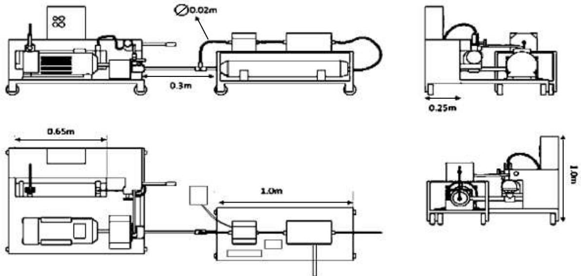
Figure 3.6: Orthographic view of test rig
