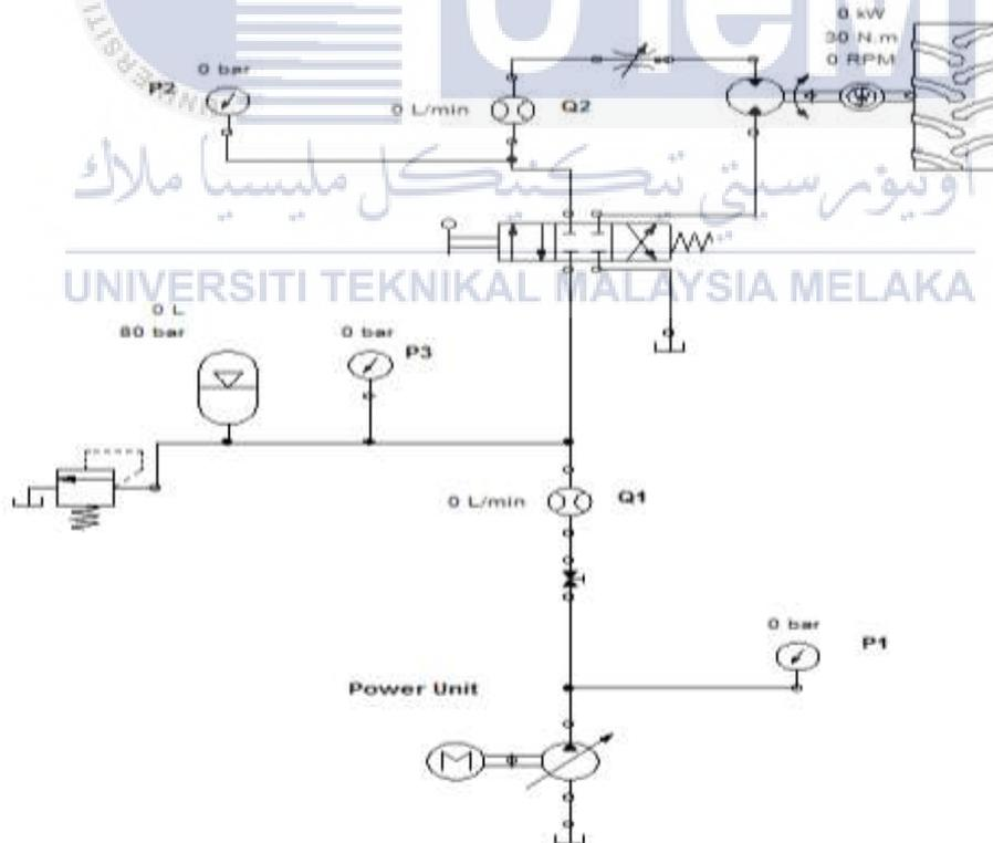
Figure 3.4: Diagram propulsion drive system
