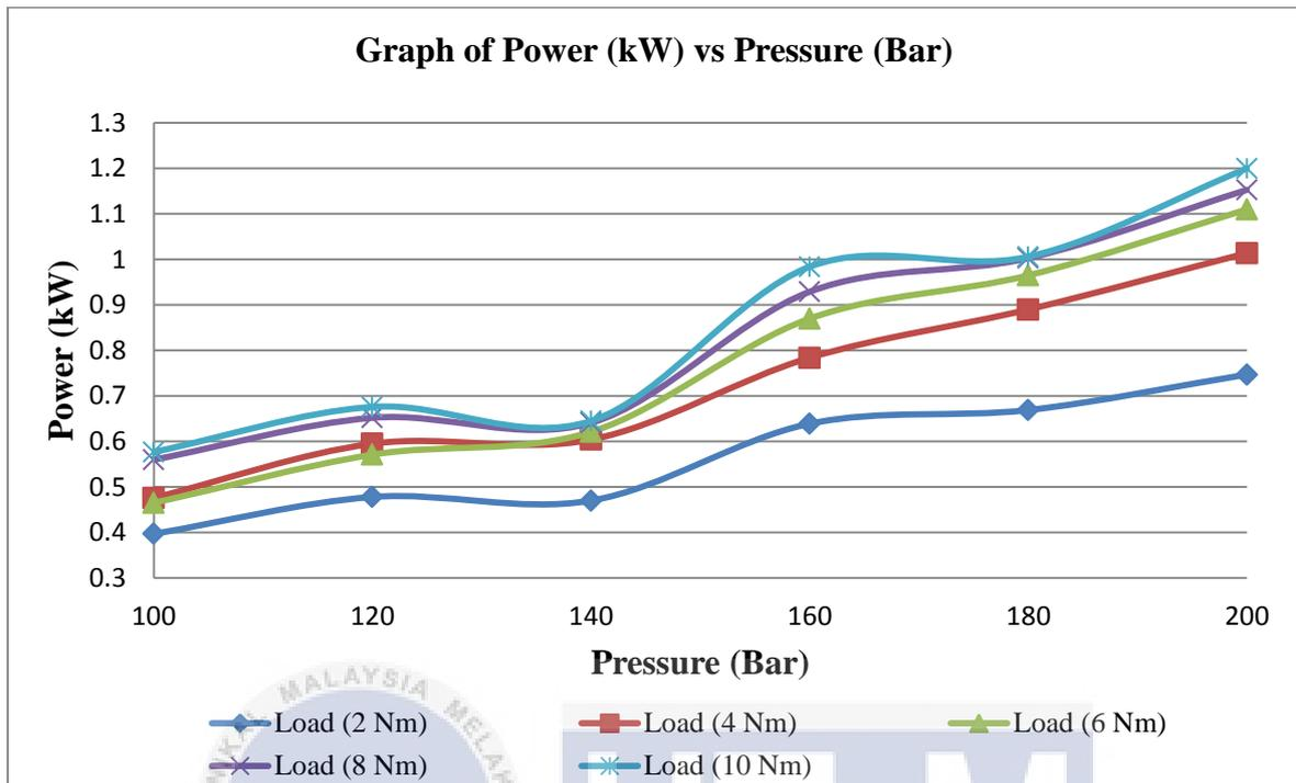
Figure 4.8: Effect of pressure change to the power
