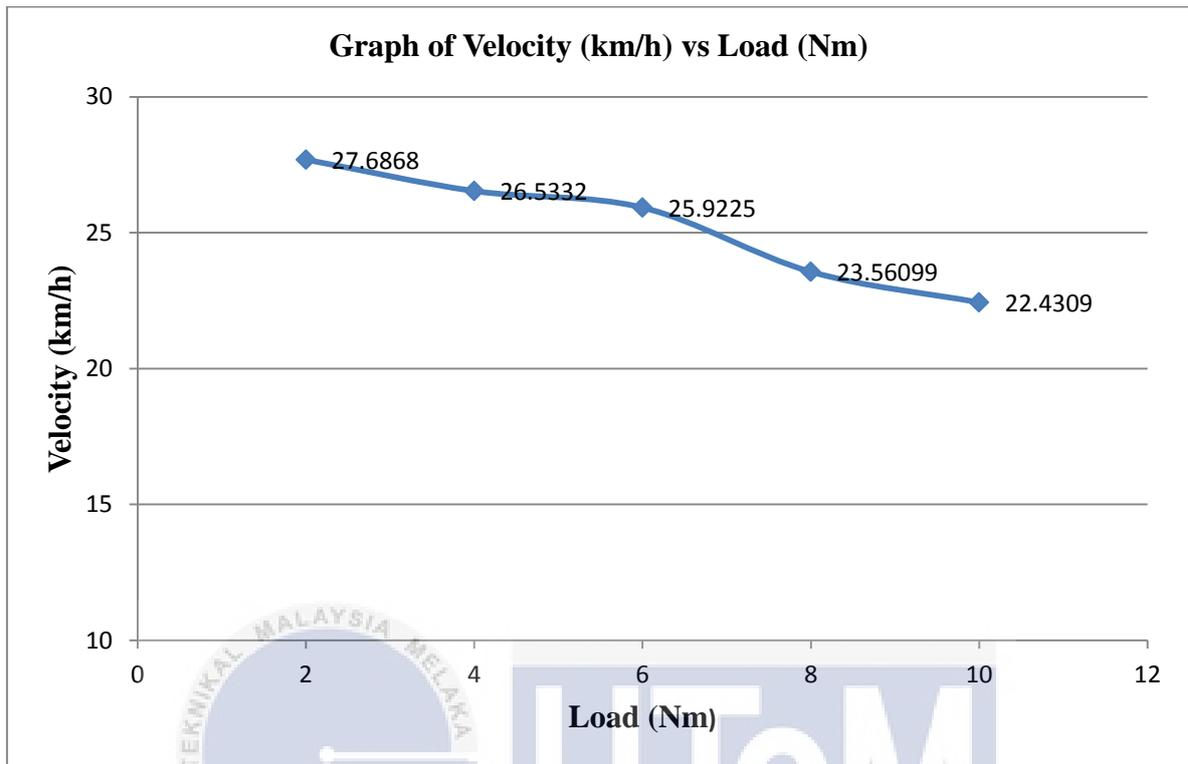
Figure 4.9: Effect of load system to the velocity at constant pressure 200 bar
