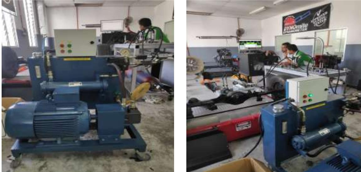
Figure 3.15: Power unit of hydro-pneumatic control the different pressure
