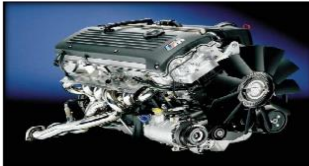
Figure 2.13: BMW's S54 inline-6 engine, which uses a gray cast iron engine block (Hieu Nguyen, 2005)
