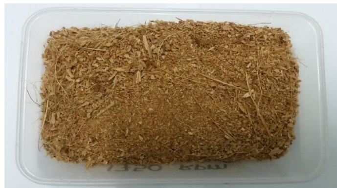
Figure 5.12: Coco crushed quality at 4500 RPM
