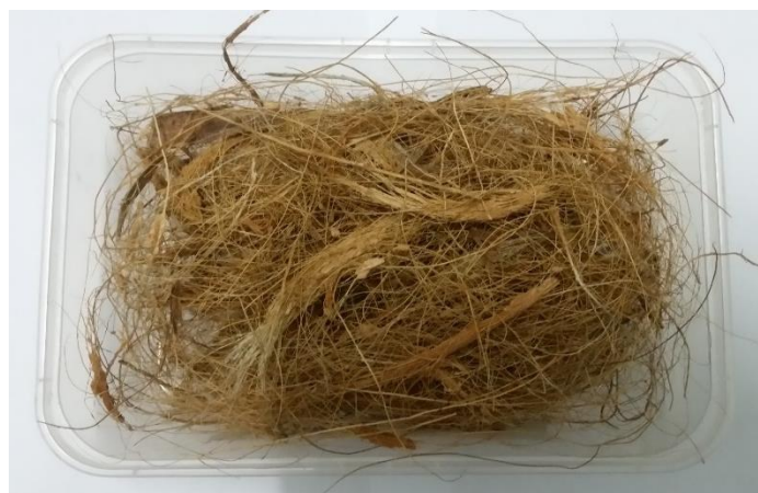
Figure 5.15: Coco fiber crushed quality at 4500 RPM
