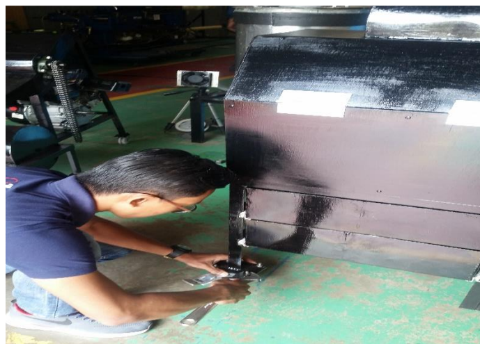
Figure 4.45: Assembling caster wheel with machine using bolt and nut
