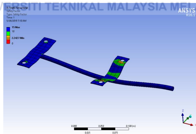
Figure 5.8: FEA safety factor for the adjuster part
