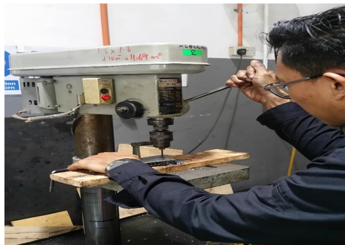
Figure 4.40: Drilling process using table drill
