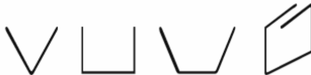
Figure 2.4: Cross-section of gutter (from left to right), V-shaped gutter, Square gutter, Trapezoidal gutter and a Wrap gutter design.
