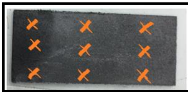
Figure 4.1: Nine different points on surface of sample
